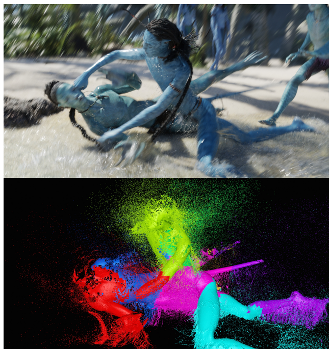
Fig. 1. Fighting kids . For a scene from Avatar: The Way of Water (top) a sparse particle-in-cell splashing water simulation with surface tension and viscosity (bottom) [Stomakhin et al. 2023] and peak total memory consumption of ~500GB has been split into 8 ranks (indicated by colors) using our Power partitioner. Top image from AVATAR: WAY OF WATER ©2022 20th Century Studios, Inc. All rights reserved. Bottom image © Wētā FX Ltd.
